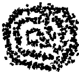
FIGURE 2 Top view of the MD box for a nanowire shown in Figure 1. Here and in Figure 3 the whole thickness of the wire along its axis is shown after 7.1 ns of simulation.
